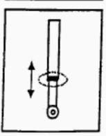
PACKING EFFECT A situation where the forks or shock, become captive at a compressed range of their travel, due to excessively slow Rebound damping, and it's effect as the bike travels over a series of contiguous bumps on the road surface.
